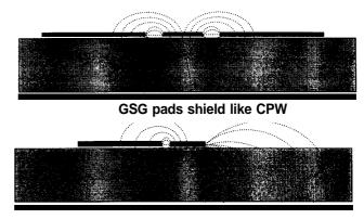
GS pads fringe to the ground plane or chuck
