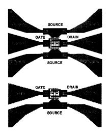
Figure 11. Microwave probe contact patterns. The Ground-Signal-Ground (GSG) pattern has higher performance than the Ground-Signal (GS/SG) configuration.
