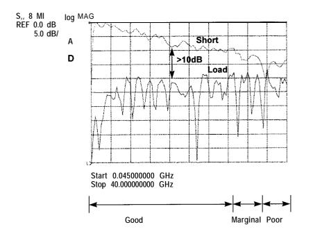
Figure 20. The relative magnitudes of uncorrected measurements of a short and a load provide a good check on proper system function.
