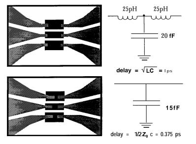
Figure 16. Improper probe placement will impact the electrical behavior of a measured standard. Use of alignment marks to set probe separation and reasonable care in placement will provide good results.
