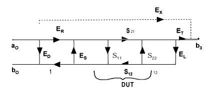
Figure 17. Signal flow graph of the full two-port VNA error model without switch corrections. The forward stimulation case is shown, a similar error model is **used** for reverse stimulation.
