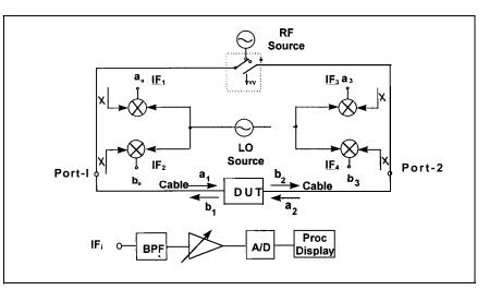
Figure 1. Main hardware blocks in a Vector Network Analyzer (VNA).
