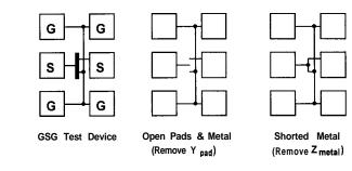
Figure 12. Pad Parasitic Removal structures.
