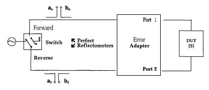
Figure 4. Error model for a typical network analyzer. All errors are modeled by an error adapter in front of an otherwise perfect system.
