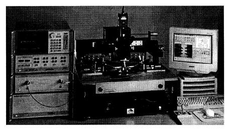
Figure 2. A typical RF device characterization setup is shown above. On the left is a vector network analyzer, in this case an Agilent 8510 system. Cables from the test set ports route over the probe station to a pair of microwave probes which are aligned through the microscope or camera system onto calibration substrates and test devices. The right side of this picture shows the PC that controls the prober and runs the calibration and measurement software.
